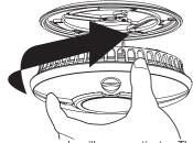
The power pack will now activate. The red LED on the front of the alarm should flash approximately once every 45 seconds to show that it is active.
